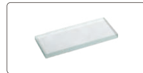
50mm reading scale (check magnification accuracy)
